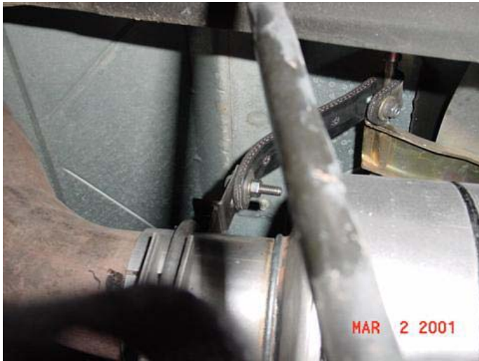
Use standard muffer hanger for rear muffer support details. Stock muffer hanger to be removed and welded to the Walker muffer.
