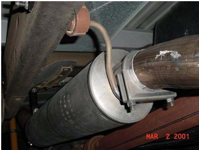
Front mount details, showing the muffler hanger, removed from the stock muffler and welded to the Walker muffler. Also shows the position of the relocated front muffler hanger bracket. The stock front muffler hanger bracket, that was relocated forward, about 12", to support the longer Walker muffler. Use existing bolt hole in the frame.
