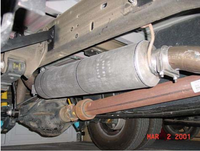
Walker #21470 'Big Truck' muffler installed
